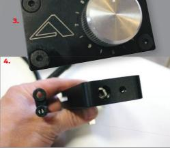
3. The custom billet controller is installed inside the cab somewhere on the dash within easy reach of the driver. With 10 clicks on the knob, you have complete control of the pump's output. Lower settings will mean lower fuel output, so better smoke control and fuel mileage, while higher settings allow for more rack travel and maximum fuel output for the drag strip and dyno.
